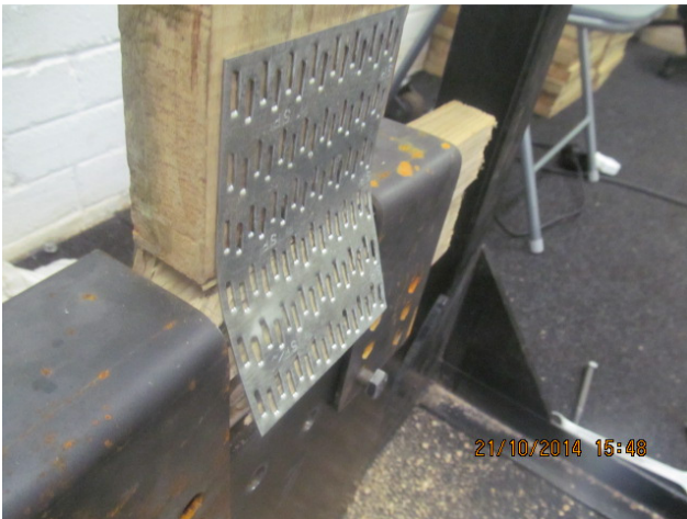
Anchorage perpendicular test failures
