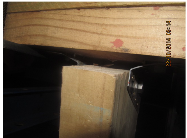
Truss Hanger tests failures
