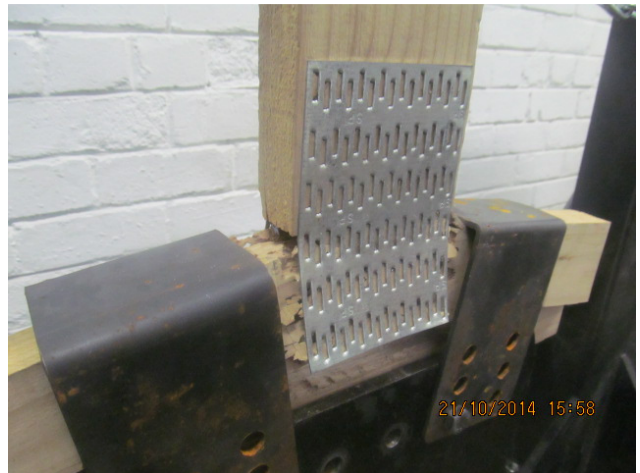
Anchorage perpendicular test failures
