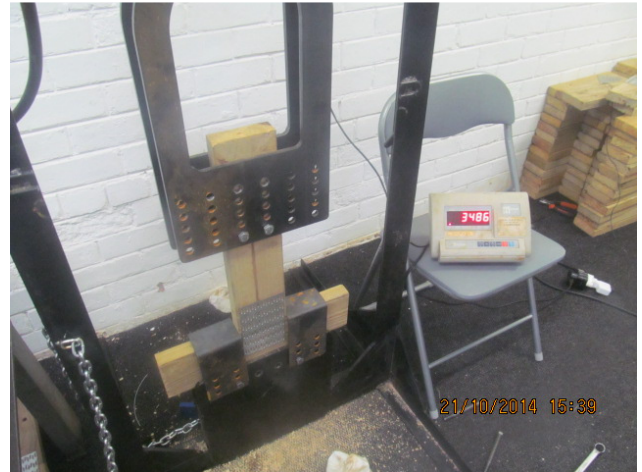
Anchorage perpendicular test failures
