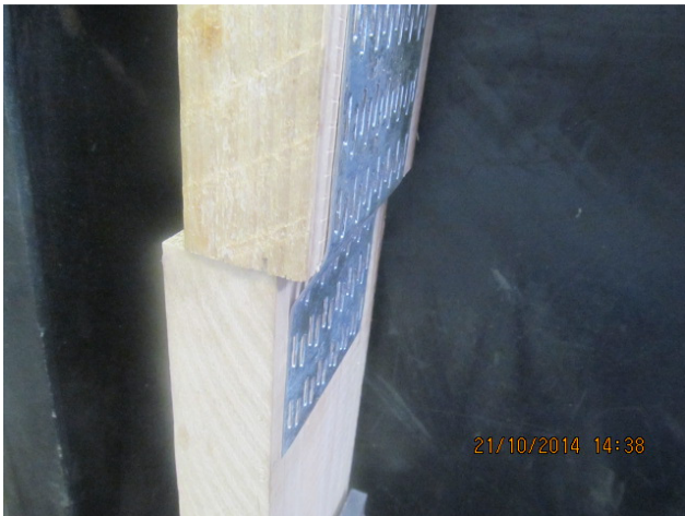
Compression strength test failures
