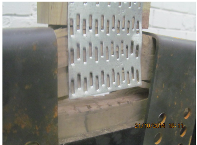
Anchorage perpendicular test failures
