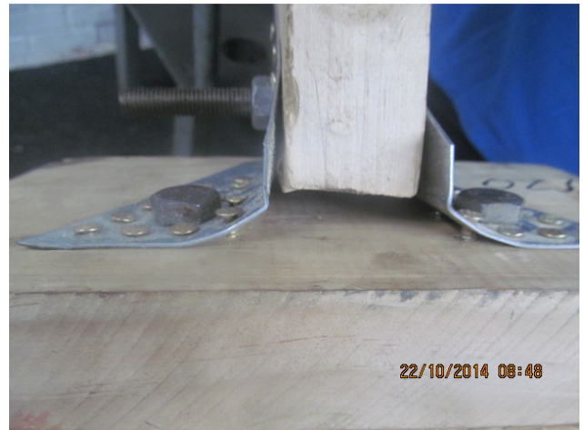
Truss Hanger tests failures
