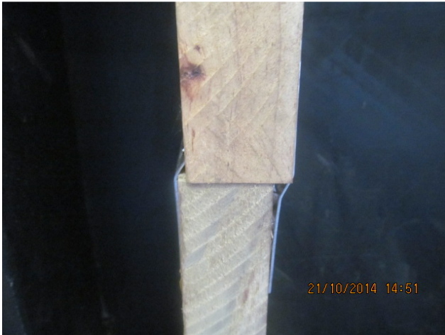
Compression strength test failures
