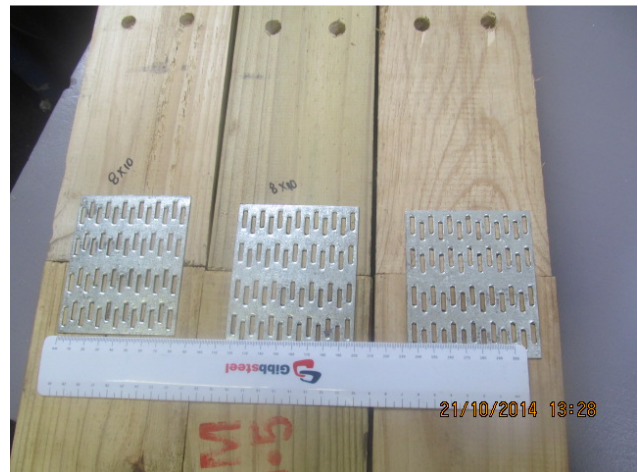
Nail plates of various sizes joining timber
