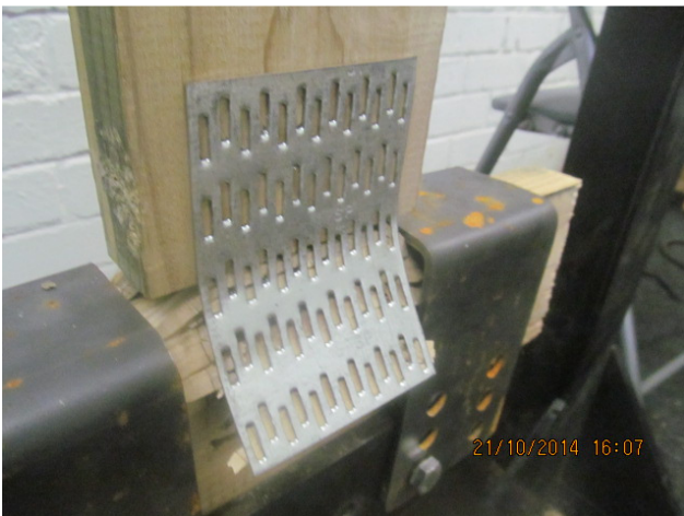
Anchorage perpendicular test failures
