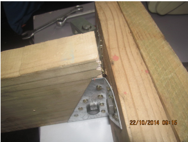
Truss Hanger tests failures
