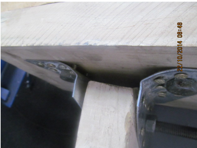
Truss Hanger tests failures
