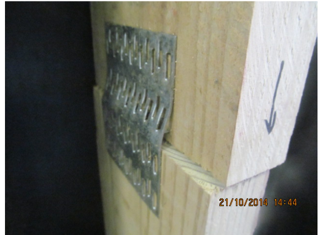
Compression strength test failures
