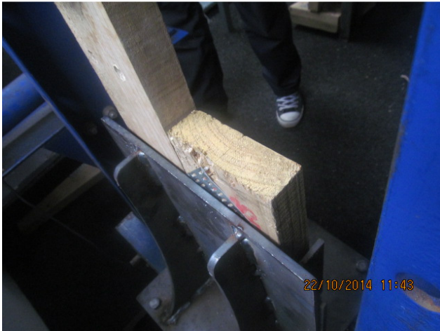
Shear strength test failures
