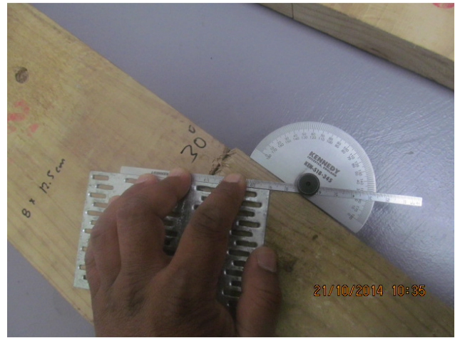
Nail plates of various sizes & angles joining timber
