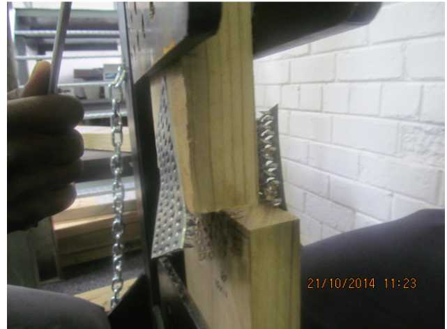
Tensile strength test failures
